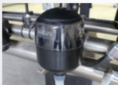
Electronic Milk Meter Real-time milking data to monitor performance
