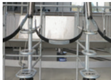
Cow Restraints Restrain cows automatically within the stall
