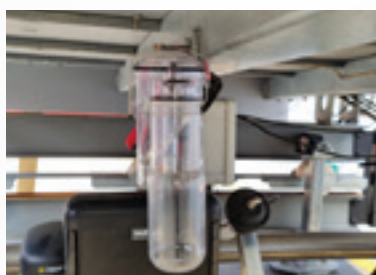
WMS Sampler Takes samples for accurate milk analysis
