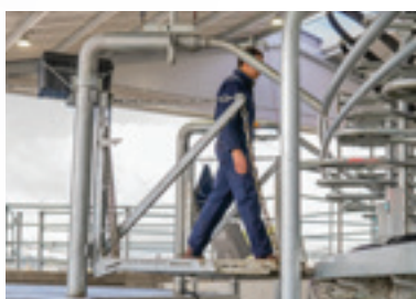
Drop Down Vet Platform Used for when treating animals on platform
