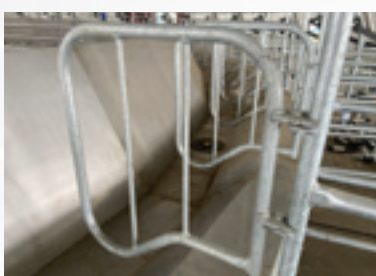
Head Dividers Prevents "feed robbing" between stalls
