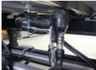
Vortex Shut Off Valve High performance milk shut off value
