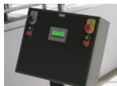
Platform Operator Console - Cups Off Second console for convenience at cups off
