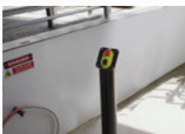
Platform Operator Console - E-Stop Can be activated in case of an emergency
