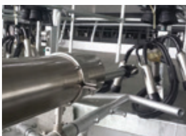
Waikato Spray Arm Automatic teat spraying for fast rotaries
