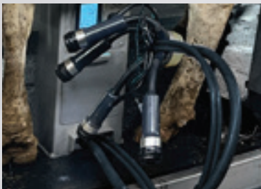
320HP Milking Cluster Ergonomically designed, lighter weight cluster
