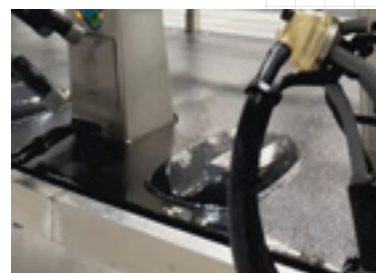
Dry Edge / Stainless Perimeter Rail Allows water to drain away from the operator
