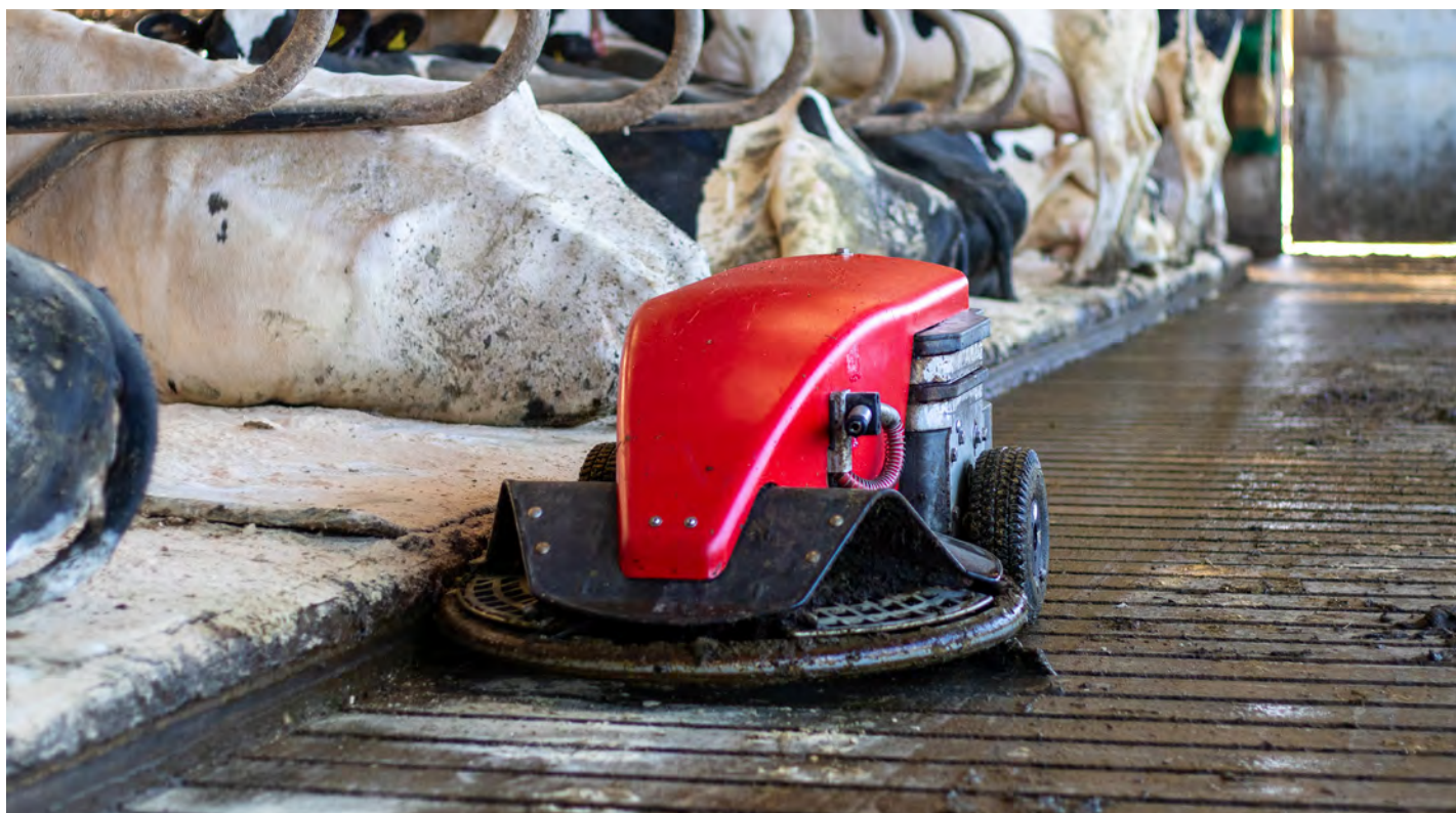
A Lely Discovery 120 is used to clean the floors. It has saved two hours daily scraping
